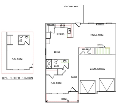
FIRST FLOOR PLAN (SCALE 1/8"=1'-0")
